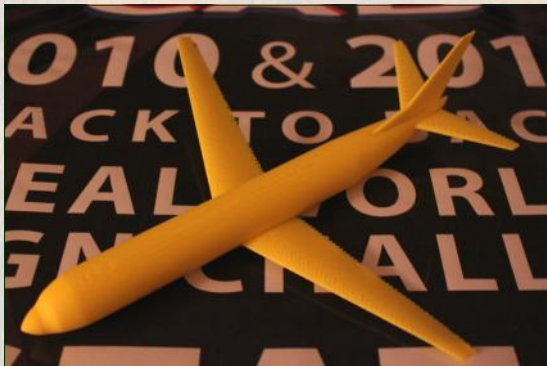
A plastic model of the MCAD 737 designed by students of Jim Mandl '90. The plane is made from ABS plastic and was created by a Dimension 3D printer in the Pre-Engineering and CAD classroom.
